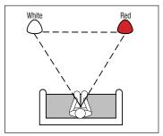
The front speakers should be placed the same distance from each other as they are from the listening position. They should be placed at about the same height from the floor as the listeners' ears will be.
